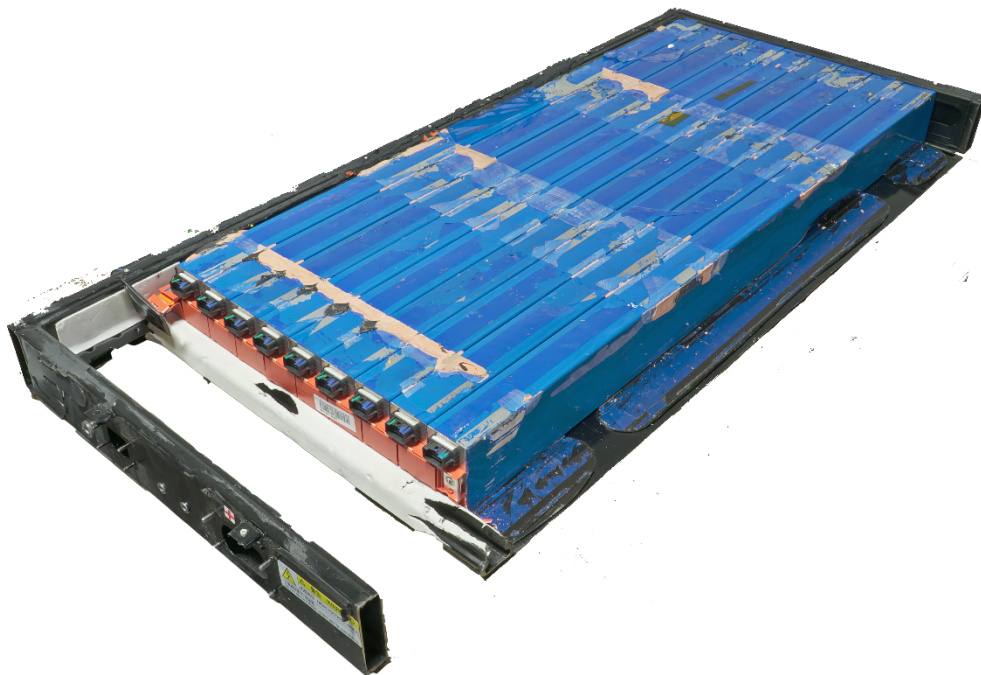
Fig. 5 "Cell to pack" example (BYD Blade); Pictures from FEV Benchmarking
