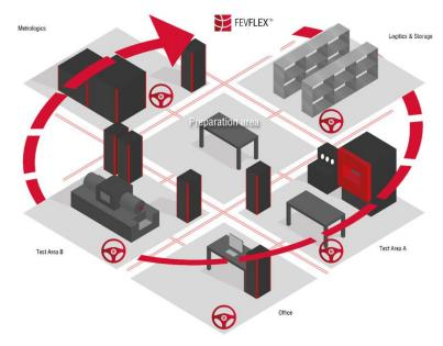
FEVFLEX™, FEV's information system, manages the flow, processes and data of a testing project. MORPHEE®, the FEV automation system, monitors equipment and test beds of the testing center – Source: FEV Group
